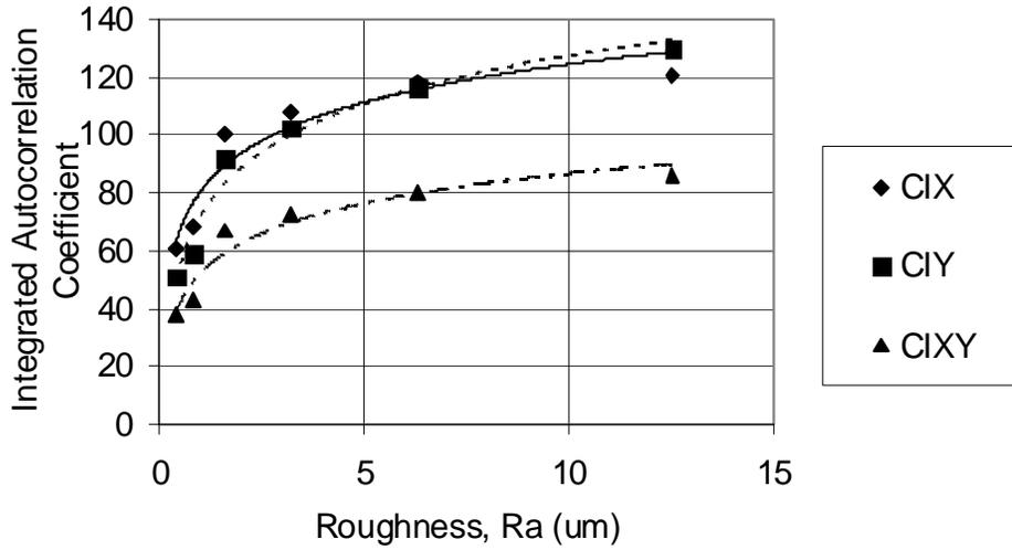
Figure 3.1: Graph of Integrated Autocorrelation Coefficient Vs Roughness
